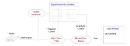
Audio signals from the radio are band-pass filtered to select the particular signal of interest. In most CW listening situations, more than one signal is audible within the listening band. This filter helps to select one signal for decoding.
